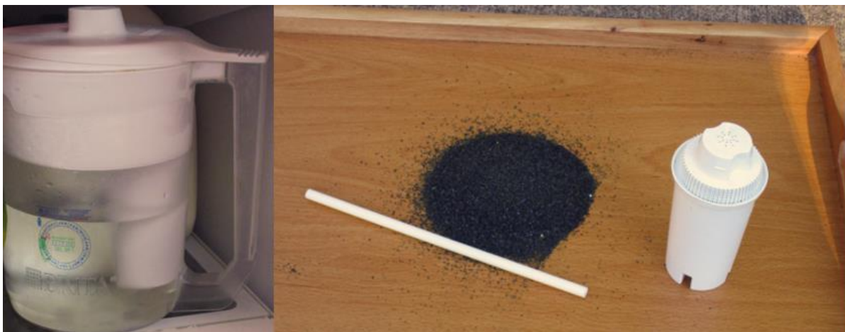
A Brita Home Water Filtration system with pitcher of purified water and carbon adsorber used inside the water filter with a straw for scale is shown. This is a simple carbon adsorber process.
